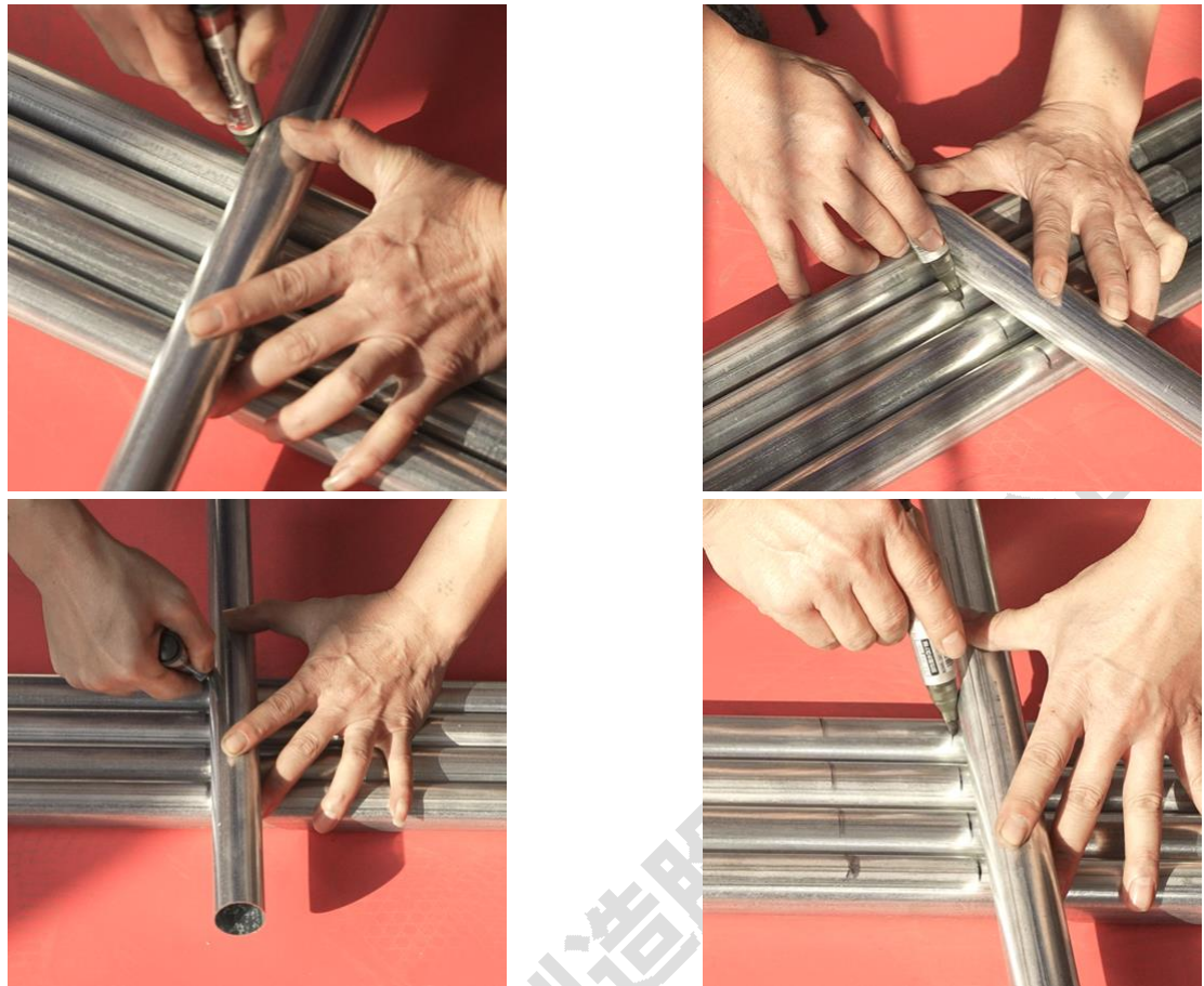
底部并齐，四根钢管做同样标记，另四根同样操作 make the bottom side same line, the same marked length for 4 pipes, same length size marks
